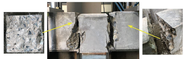
(b) 100% replacement with treatment(R-10-Y1, P_f : 441.6kN)
