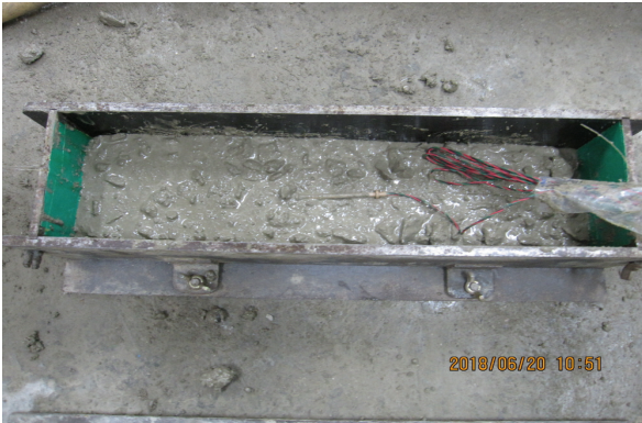
Fig. 4. Photos of pouring concrete for autogenous and drying shrinkage test
