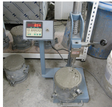
Fig. 2. Setting time investigation in test
