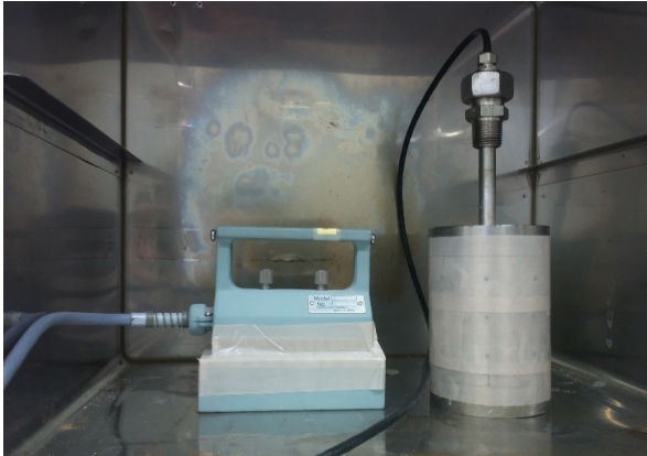
Fig. 2. Temperature measurements of the compacted bentonite.
