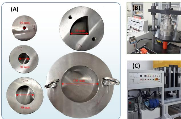
Fig. 3. Photos of dies with diameters of 1, 3, 5, 10 cm and one quarter of 10 cm-diameter circle (A), press for dies in photo of (A) (B), and large press for die of one quarter of 40 cm-diameter circle (C).
