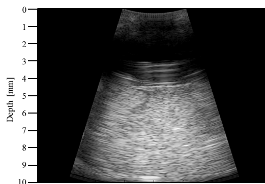
Fig. 2. Ultrasound image of the BSA phantom before HIFU exposure.
