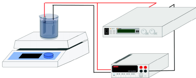
Figure 1. Schematic diagram of the instrument used in the experiment. The potential is applied by DC power source (ODA-EX300-4) and current is measured by digital multimeter (KEITHLEY 2000). The reaction temperature is controlled with a hot plate.
