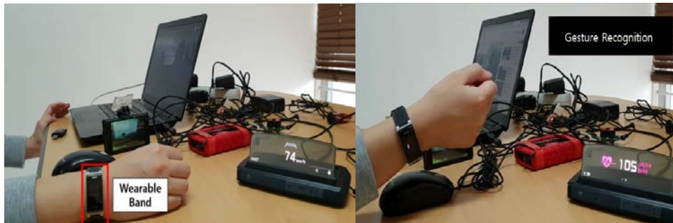
Fig. 7. Implementation and test environment for the gesture recognition method: (a) system set up; (b) gesture recognition test
