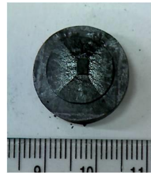
Fig. 7. Digital image of a melt-processed Y1.8-carbonate with Y1.8-SCI buffer pellet. As-pressed Y1.8-carbonate compact has been melt-processed without any prior heat treatment before a melt process.
