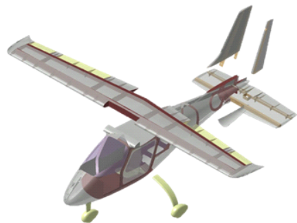
Fig. 12. Structural configuration of OPNAV
