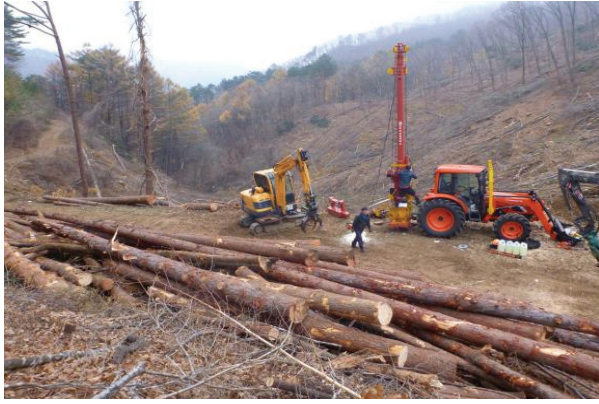
Figure 1. Tree-length logs extraction using HAM300 and small-shovel.
