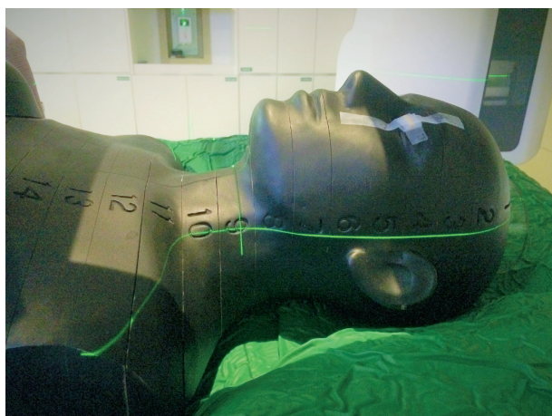
Fig. 3. Absorbed dose measurement of Rando Phantom
