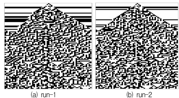
Fig. 7. True random data generation results of CARR-TRNG operated with the same initial value (black and white denote ‘1’ and ‘0’, respectively).
