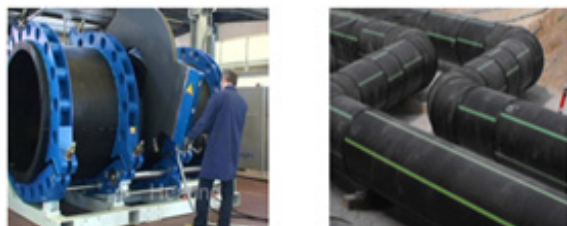
Figure 1. Heated tool bonding of large diameter HDPE pipes. (a) Butt fusion equipment [1] and (b) butt fusion joints in HDPE pipe [2].
