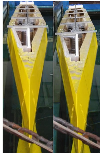
[Figure 4] intact Condition(Left), Damaged Condition(Right)
