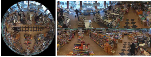
Fig. 1. 360-degree and calibrated views of a commercial fisheye lens camera[3].
