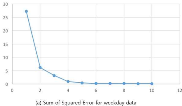
Fig. 6. (a) Graph of Sum of Squared Error for weekday data (K=4 by 'elbow' method), (b) Weekly Schedule Set-point Table learned from User's usage pattern.
