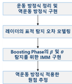
Fig. 1. A process of launch point estimation of a high-speed vehicle
