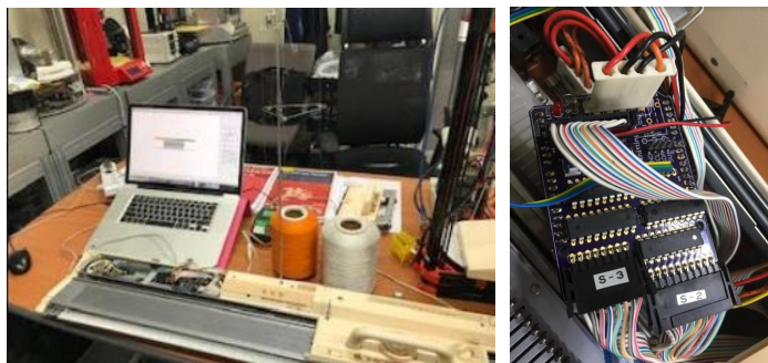
Figure 1(a). Open source knitting machine upgrade production, Figure 1(b). Ayab circuit board
