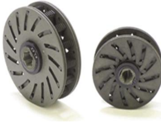
Figure 2. Structure of centrifugal belt pulley CVT
