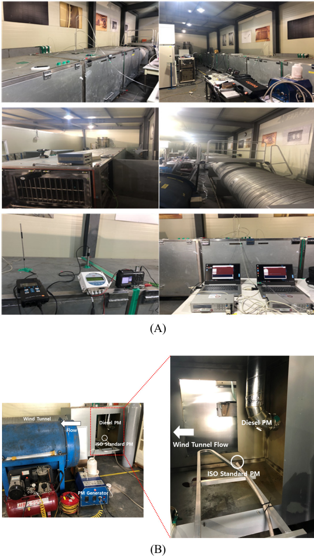
Figure 4. Picture of wind tunnel system (A) and PM spray experiment equipment (B).
