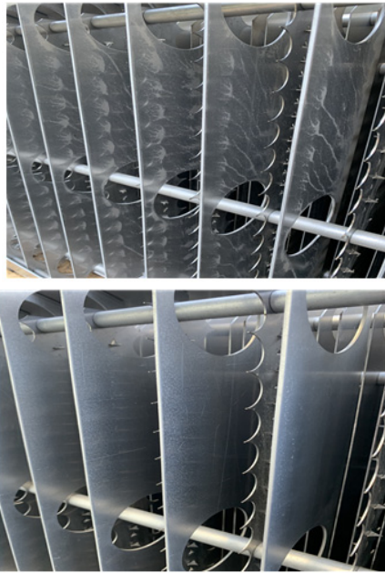
Figure 12. Picture of before and after by washing using tap water (top) and nano-bubble (bottom).
