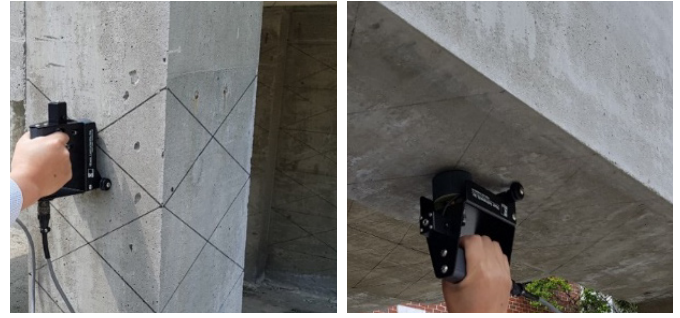
Figure 4. Experiment of impact echo method
