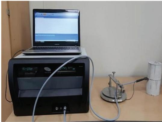
Fig. 8. Test setup of thermal conductivity
