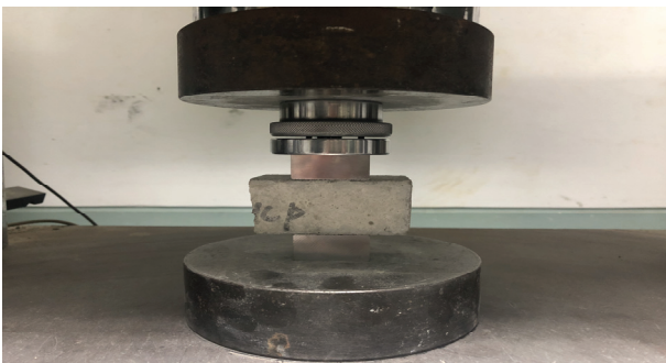
Fig. 4. Reloading test of specimen with pre-compressive load
