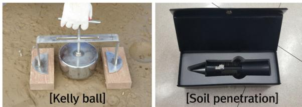
Fig. 4. Kelly ball drop and soil penetration equipment
