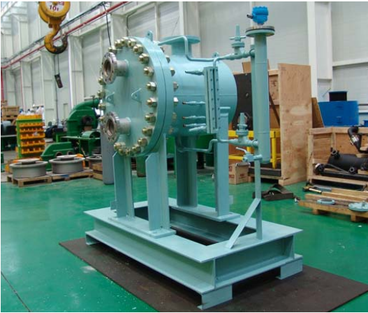
Fig. 10. P&SHE for flooded chiller system.
