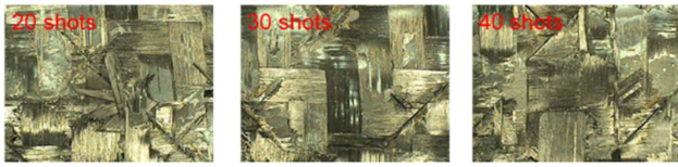
Fig. 10. Bonded surface of fractured specimen in shear test according to the number of laser shots
