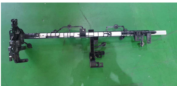
Fig. 4. A Cowl Cross Member with multi-material type (polymer+ aluminum bar)
