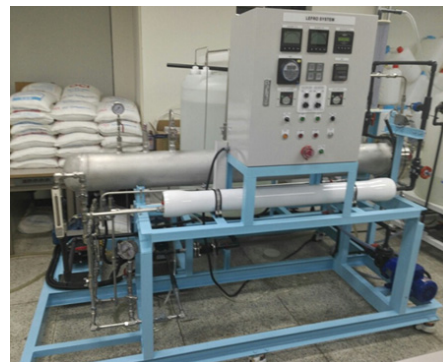
Fig. 1. Schematic and picture of high pressure membrane system used in this work.
