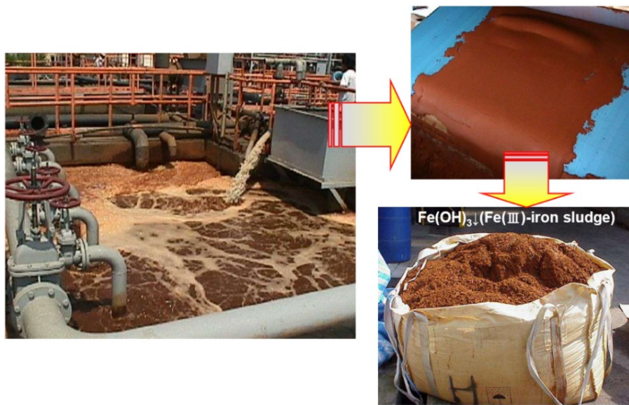
Fig. 3. Production of iron sludge after the Fenton process (Source: Prof. Y.H. Huang, National Cheng Kung University, Taiwan).
