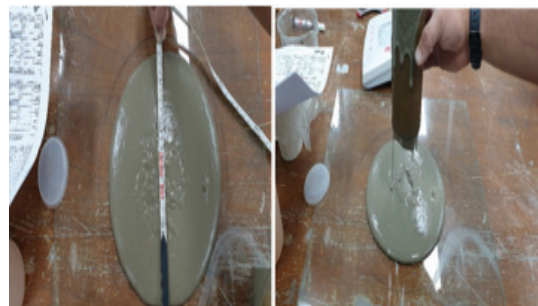
Fig. 2. Mini-slump spread for pumpability.
