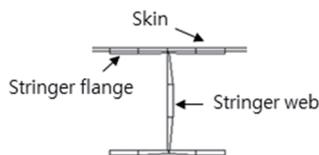
**Fig. 2** Modeling Concept for Contact Area between Skin and Stringer
