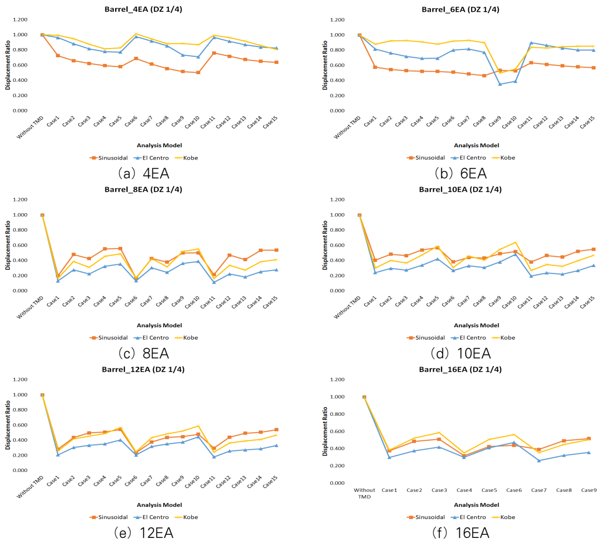
〈Fig. 6〉 Maximum vertical displacement ratio of earthquake wave (Barrel type 1/4 point)
