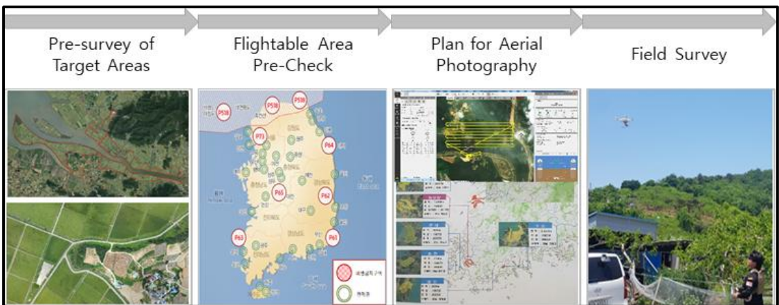
Fig. 1. Procedures for aerial photography using unmanned aerial vehicles.
