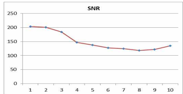
Fig. 8. Measurement value for SNR to the Flow Rate change.
