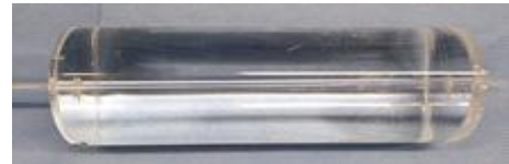
Fig. 1. Water Phantom of 3 mm vessel model.
