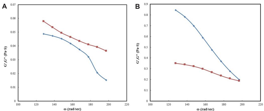
**Fig. 1. The rheological behavior lines of frequency versus storage modulus ( $G'$ ) and loss modulus ( $G''$ ). (A)** Plot of  $\log G'$  (◇),  $\log G''$  (□) versus  $\omega$  milk protein-probiotic capsule mixtures at 25°C. **(B)** Plot of  $\log G'$  (◇),  $\log G''$  (□) versus  $\omega$  milk protein-probiotic capsule mixtures at 40°C.
