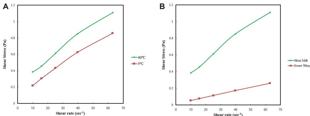
**Fig. 2. The temperature and protein source are attributed to viscosity of milk-probiotic capsules. (A)** Shear stress-versus shear rate plots of milk-probiotic capsules at 40°C and 5°C. **(B)** Shear stress-versus shear rate plots of the milk-probiotic capsules and whey-probiotic capsules at 25°C.
