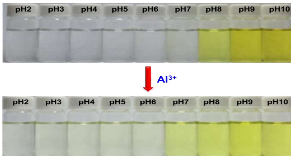
Figure 6. Effect of pH and color changes of TQC with and without \text{Al}^{3+} in normal light.
