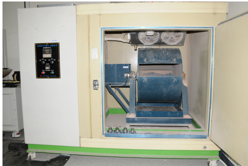
Fig. 2. LA Abrasion Tester in Constant Temperature Chamber
