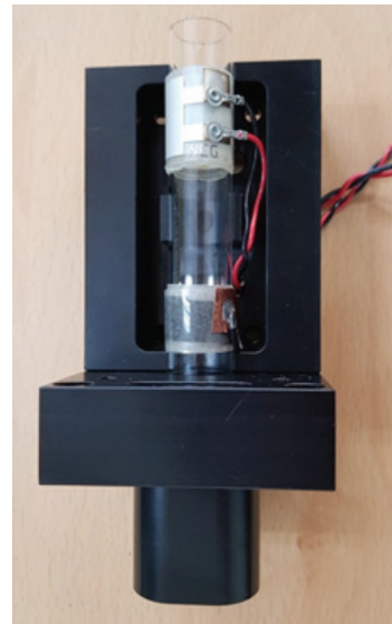
Fig. 3. Schematic diagram and view of the module developed for concentration measurement of the inorganic nutrients.
