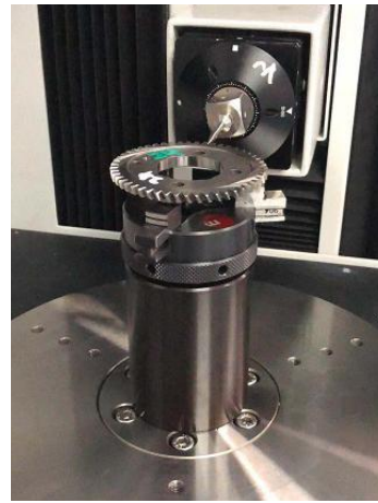
Fig. 3 Gleason metrology system for bias gear inspection
