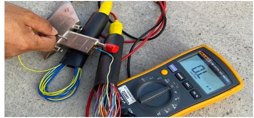
Fig. 12 First officer pitot probe resistance checked normal
