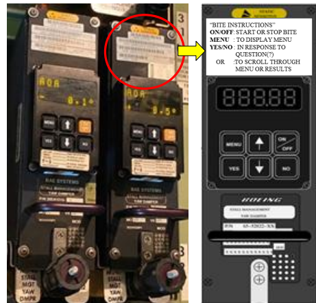
Fig. 13 SMYD(Stall management yaw damper) - AOA real data (SMYD 1: -0.1°, SMYD 2: +0.5°)
