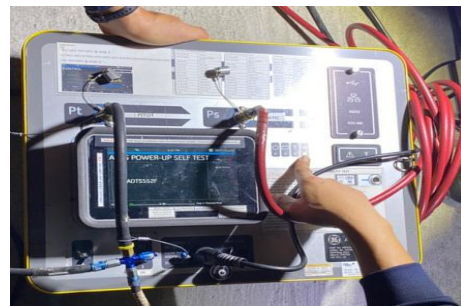
Fig. 14 Pitot probe pressure testing
