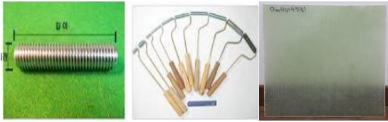
Fig. 5 Vacuum pressure : 0mmHg (hand lay-up), GFRP sheet and tools
