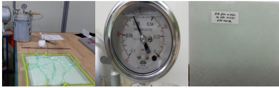
Fig. 6 Vacuum pressure: -450mmHg & -760mmHg (RTM), GFRP sheet and tools
