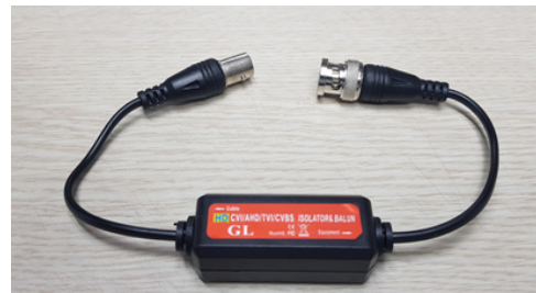
Fig. 2. In this study, a ground loop isolator (NEXT-001HDGL) was used to reduce the electrical noise generated by the HPGe detector.
