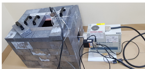
Fig. 3. Gamm-ray measurement spectrometer system (HPGe detector) of gamma-ray from the gamma ray sample.
