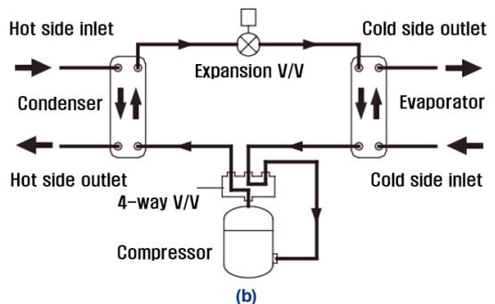
Fig. 2. Operation mode of heat pump unit (a) cooling mode, (b) heating mode
