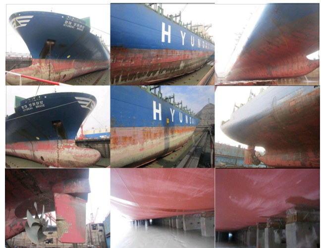
(a) Before blasting & painting
