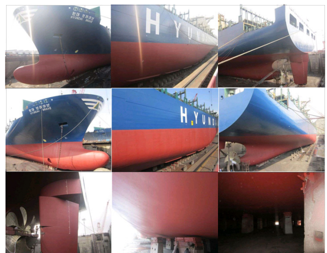
(b) After blasting & painting
