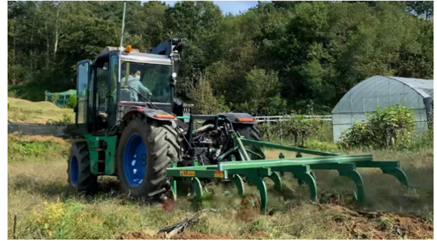
Fig. 4 Plow tillage of multi-purpose agricultural implement machinery
