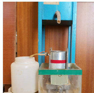
(b) Permeability test
