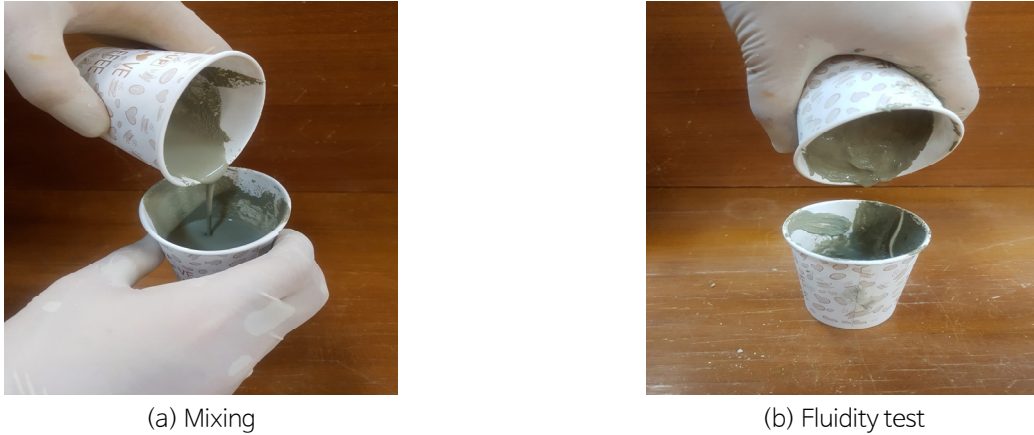
Fig. 2. Experimental fiber fluidity test of grout materials.
