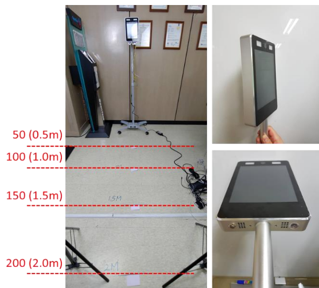
Fig. 13. Experiment space and face recognition device.
