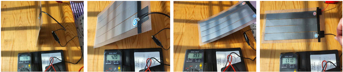
Fig. 15. Voltage level according to solar panel angle.
