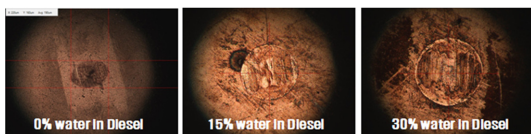
Fig. 3. Test result of wear scar test under HFRR.
