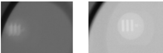
Fig. 20. Before & after autofocusing image of wide FOV at 71°C.
